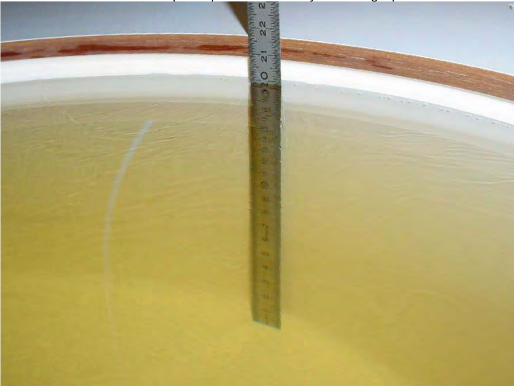
Photo 2: Liquid depth 850 MHz body simulating liquid
