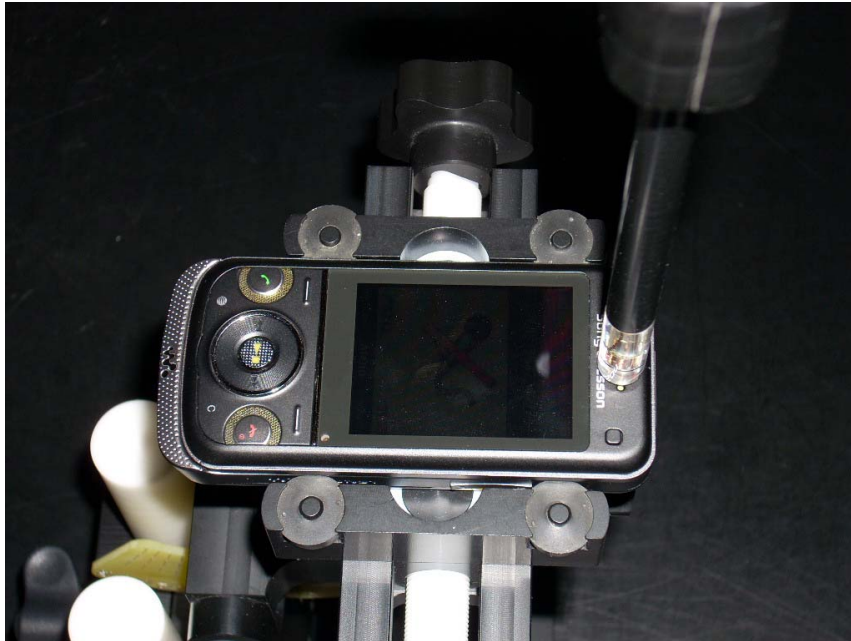
Figure 13-1 Test Setup for Wireless Device
