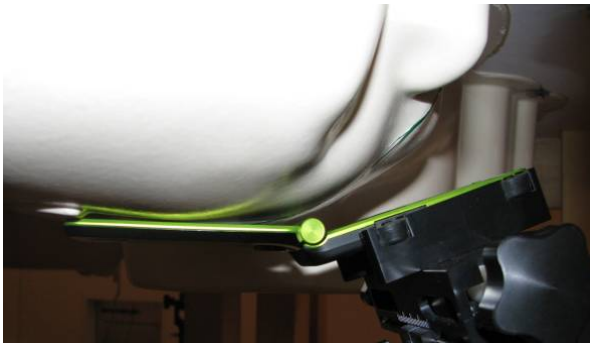
DUT position towards the head: Cheek (touch) position
