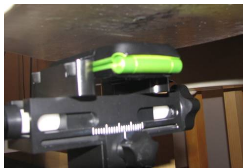
DUT in body position with 15 mm distance
