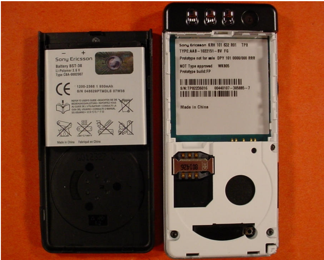
Photo 6: DUT - rear view (open) without battery
