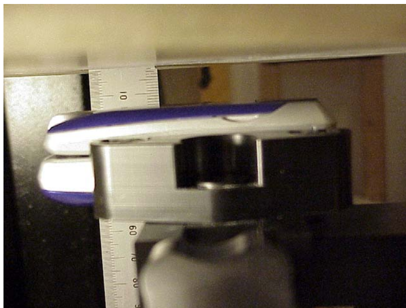
Device position against the body: Phone on 15mm from the phantom
