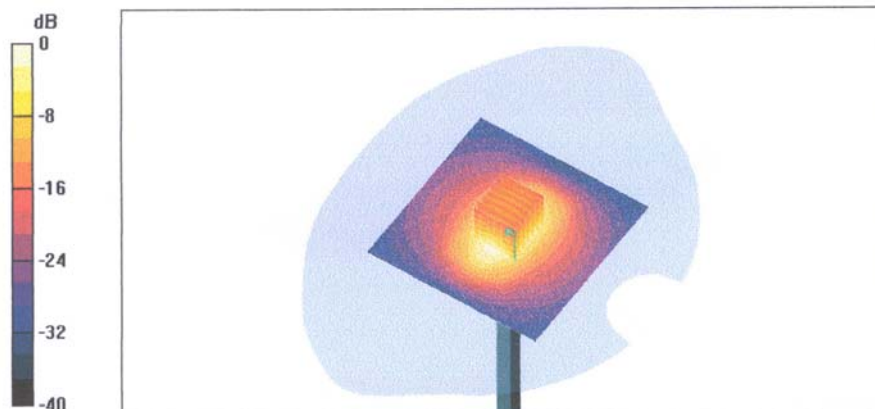
1900MHz SAR distribution of validation dipole from reference measurement with head simulating tissue
