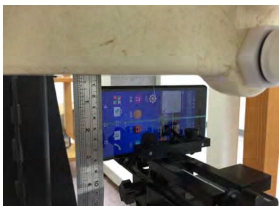
Fig.16 EUT left to flat phantom
