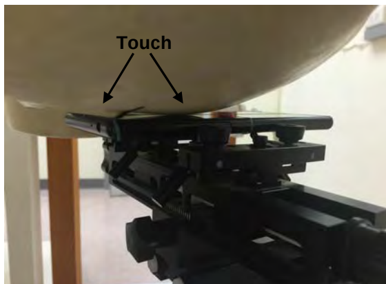
Fig.3 Right Head Section / Cheek-Touch Position
