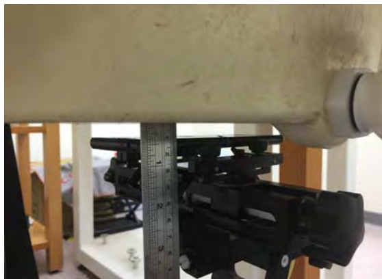
Fig.9 EUT front to flat phantom
