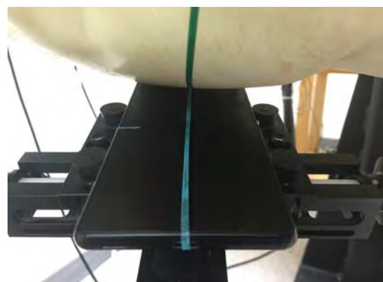
Fig.4 Right Head Section / Ear-Tilt Position(15°)
