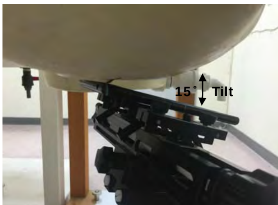
Fig.4 Right Head Section / Ear-Tilt Position(15°)
