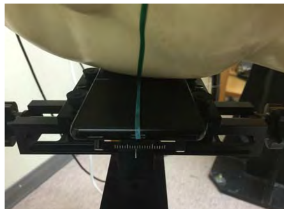
Fig.3 Right Head Section / Cheek-Touch Position
