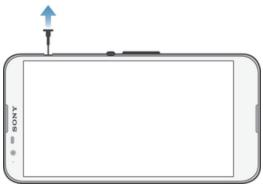
Insert a fingernail into the gap and pull out the Mobile TV antenna.
