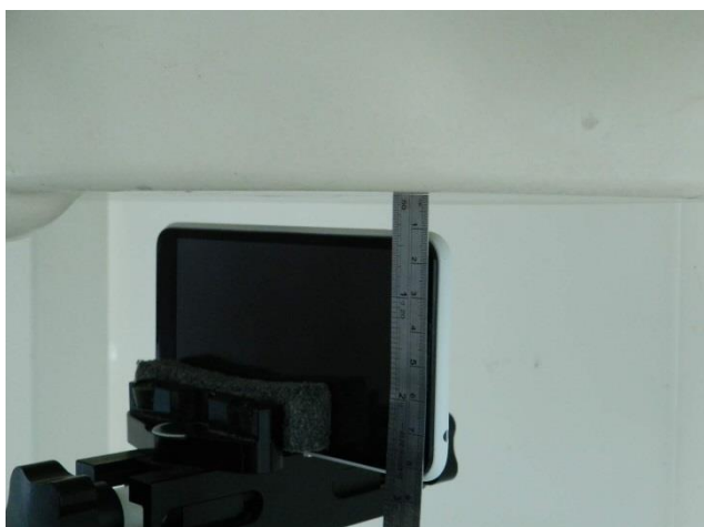
Left Side, Test Separation 1.0 cm
