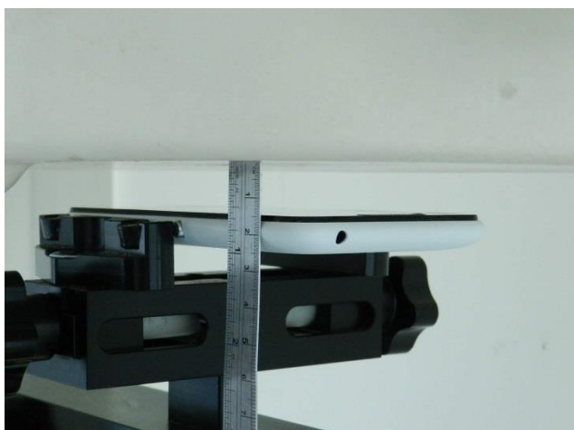
Front, Test Separation 1.5 cm
