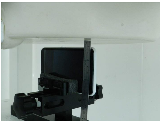
Right Side, Test Separation 1.0 cm
