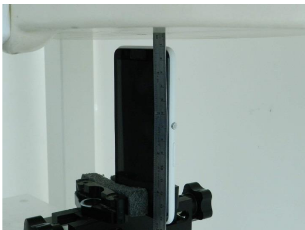
Top Side, Test Separation 1.0 cm
