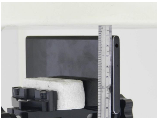
Left Side, Test Separation 10 mm
