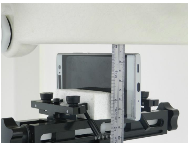
Right Side, Test Separation 10 mm
