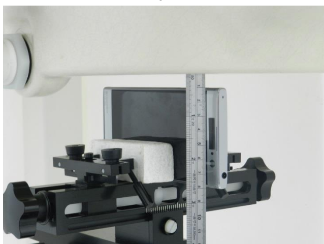
Left Side, Test Separation 10 mm
