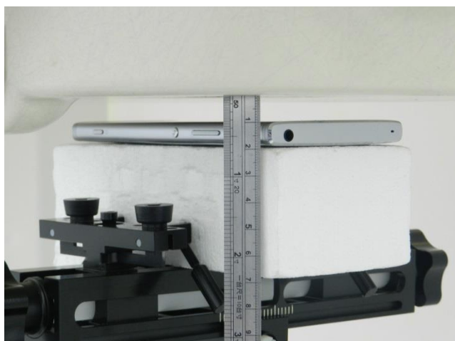
Front, Test Separation 10 mm
