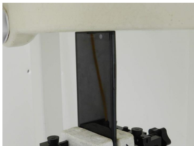
Top Side, Test Separation 0 mm
