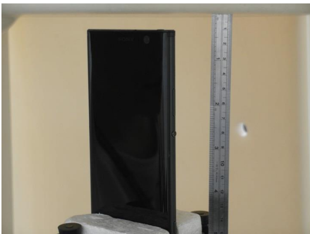
Top Side, Test Separation 10 mm
