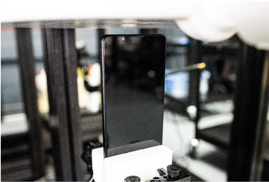
Figure J SAR Test Setup – Hotspot – Top 10mm
