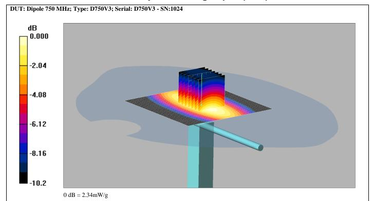
Communication System: CW; Frequency: 750 MHz; Duty Cycle: 1:1
