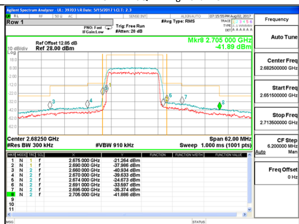
LTE B41 15MHz 16QAM High Channel FRB
