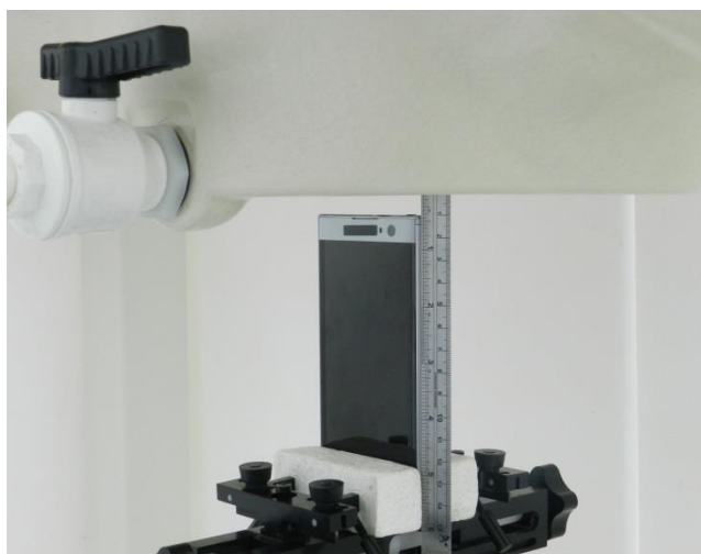
Top Side, Test Separation 10 mm
