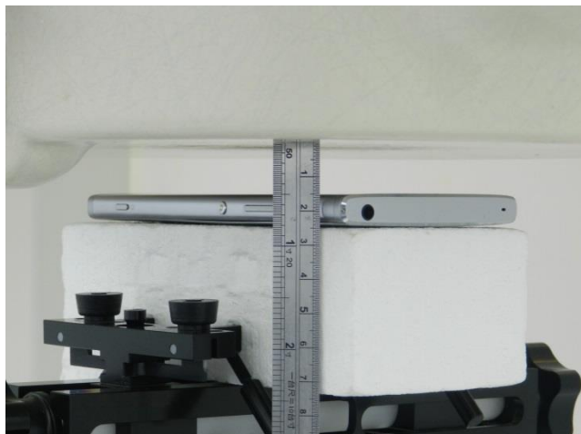
Front, Test Separation 15 mm
