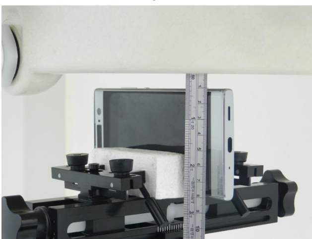
Right Side, Test Separation 10 mm
