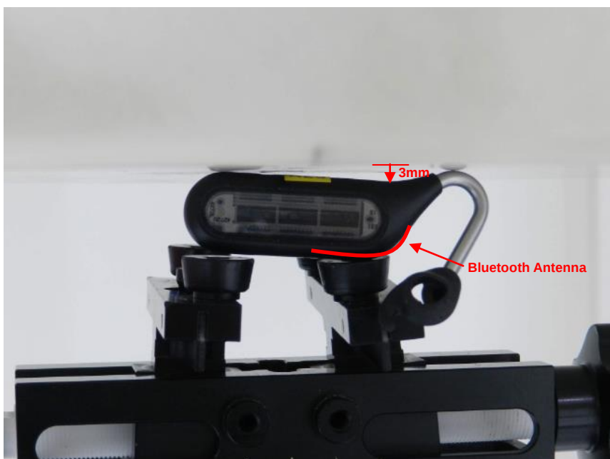
Right side (Flat phantom), additional separation introduced by the contour against a surface of the Flat phantom is 3 mm
