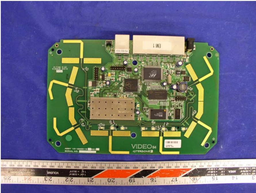
Board – Top View without Shielding
