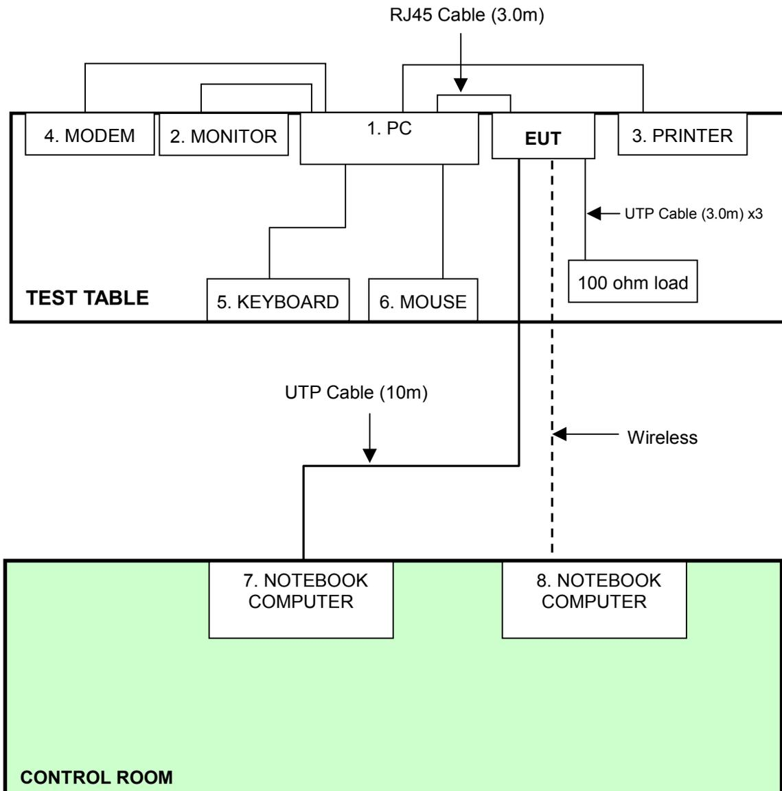
NOTE: 1. Support units 7-8 were kept in the control room during the test.
