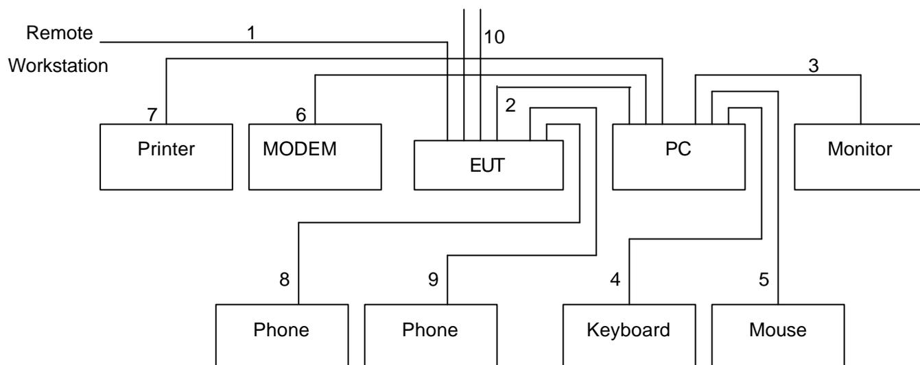
1. The RJ45 cable is connected form remote workstation to the EUT.
