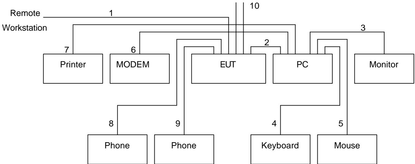
1. The RJ45 cable is connected form remote workstation to the EUT.
