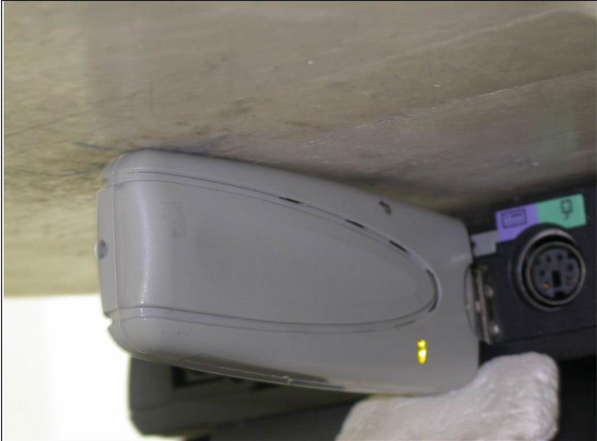
The lateral side of the EUT to the flat phantom distance 0mm
