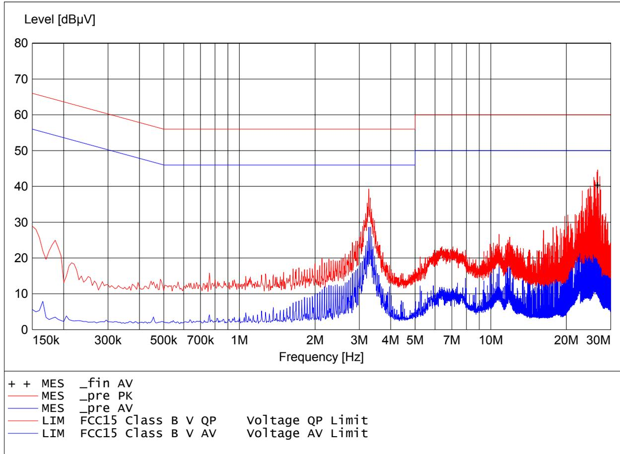
**EMI voltage test in the ac-mains according to FCC Part 15**
