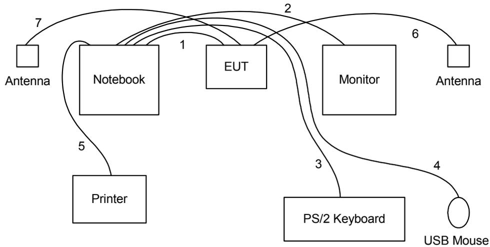
1. The TP cable is connected from PC to the EUT.
