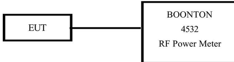
1. The output of the transmitter is connected to the BOONTON RF Power Meter.
