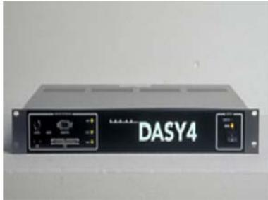
The DASY4 measurement server is based on a PC/104 CPU board with a 166MHz low-power Pentium, 32MB chip disk and 64MB RAM. The necessary circuits for communication with either the DAE3 electronic box as well as the 16-bit AD-converter system for optical detection and digital I/O interface are contained on the DASY4 I/O-board, which is directly connected to the PC/104 bus of the CPU board.
