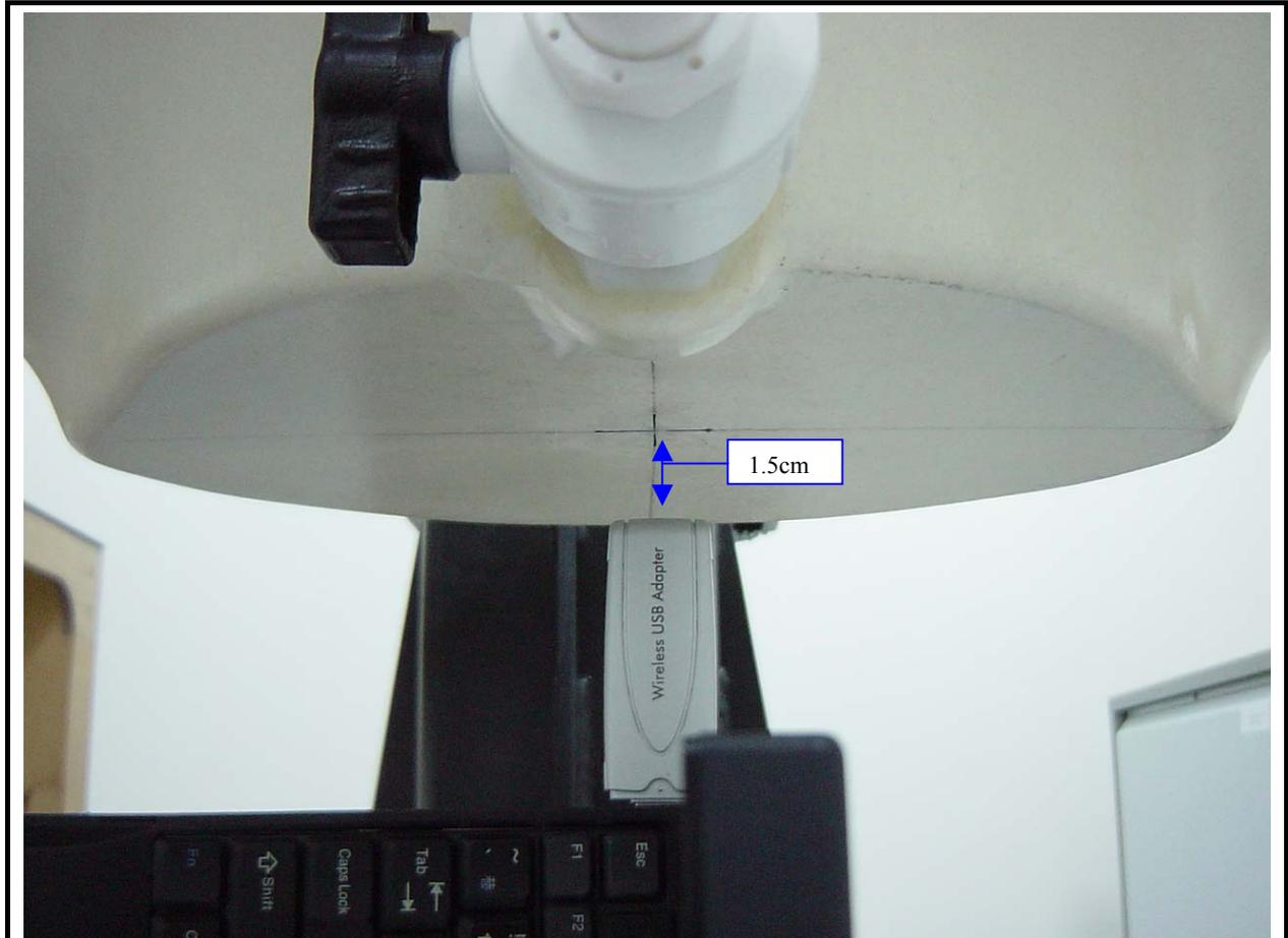
802.11b (DSSS): Duty Cycle = 100 %, Crest Factor: 1. Depth of liquid: 15.0 cm
