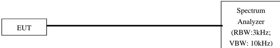
Test Configuration of Power Spectral Density
