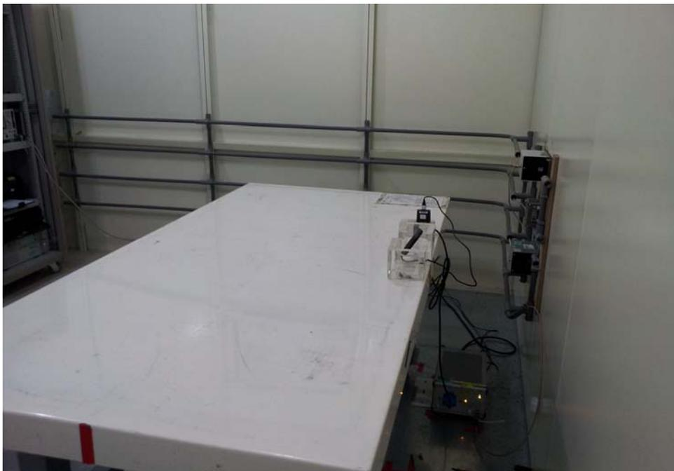
**Radiated Emissions Test Configuration:**
