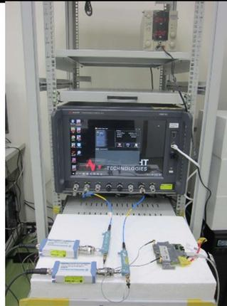
Setup for Conducted Power Test (for ENDC)
