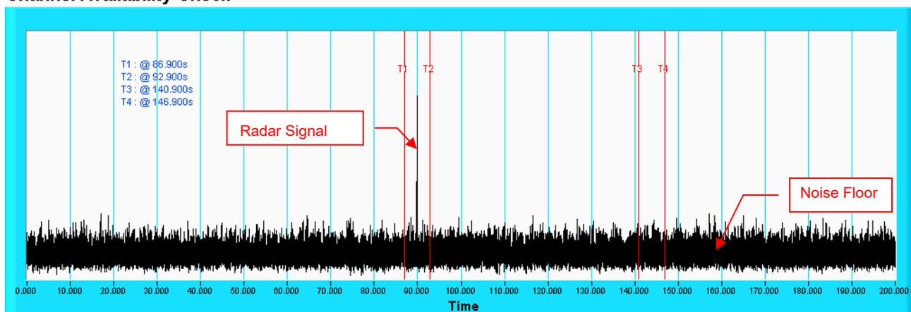
Note: T1 denotes the end of power up time period is 86.9<sup>th</sup> second. T2 denotes 92.9<sup>th</sup> second and the radar burst was commenced within a 6 second window starting from the end of power-up sequence. T4 denotes the 146.9<sup>th</sup> second.
