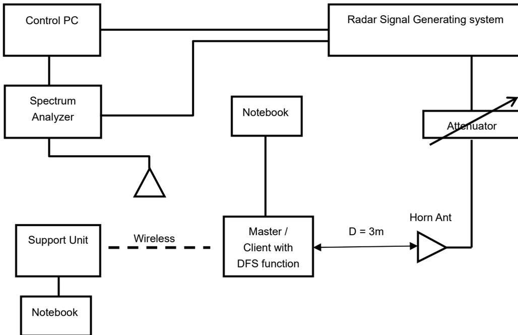
The EUT is a U-NII Device operating in Master mode. The radar test signals are injected into the Master Device.
