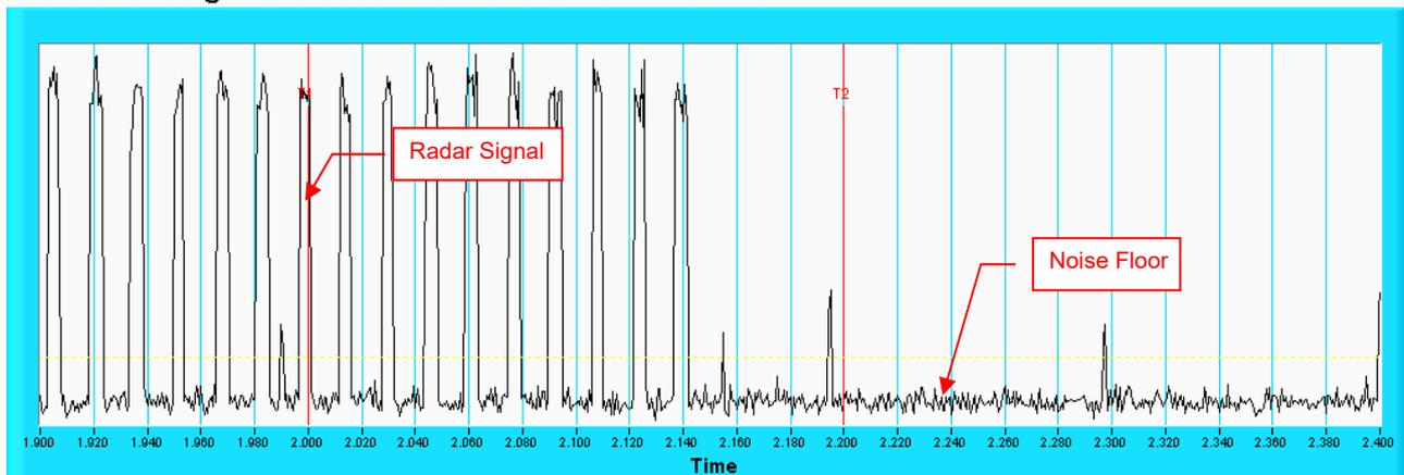
Note: Room-in of the first 500ms after radar signal applied.
