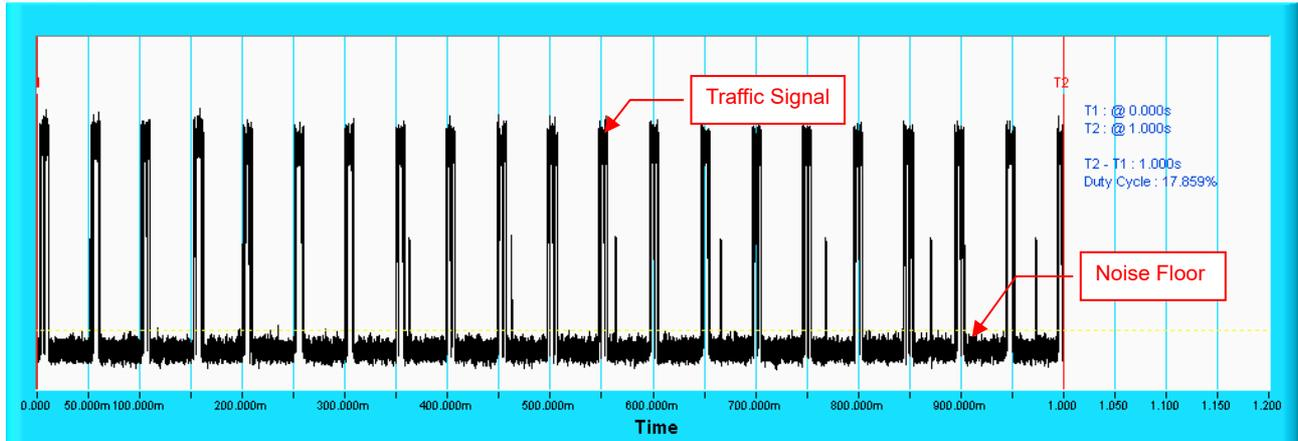
Note 1: Traffic signal: from master transmit to slave.
