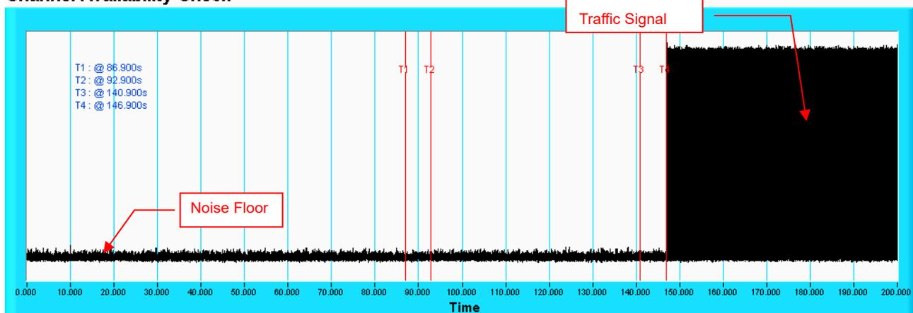
Note: T1 denotes the end of power-up time period is 86.9<sup>th</sup> second. T4 denotes the end of Channel Availability Check time is 146.9<sup>th</sup> second. Channel Availability Check time is equal to (T4 – T1) 60 seconds.
