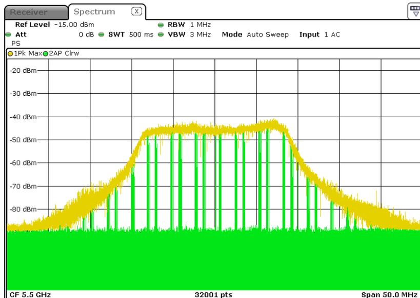
3) Radar signal is applied to the Master device and WiFi traffic signal stop immediately.
