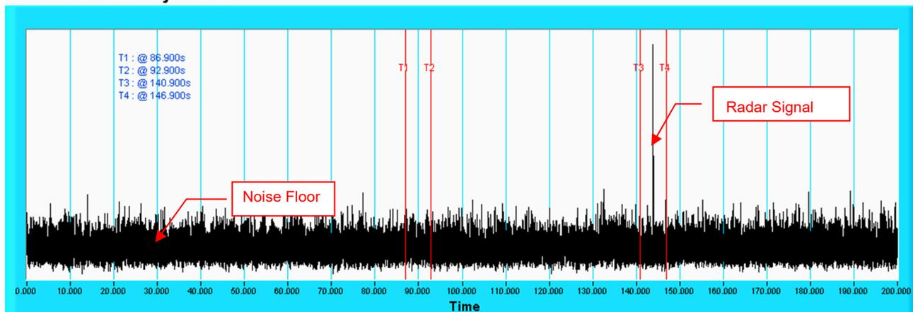
Note: T1 denotes the end of power up time period is 86.9<sup>th</sup> second. T3 denotes 140.9<sup>th</sup> second and the radar burst was commenced within 54<sup>th</sup> second to 60<sup>th</sup> second window starting from the end of power-up sequence. T4 denotes the 146.9<sup>th</sup> second.
