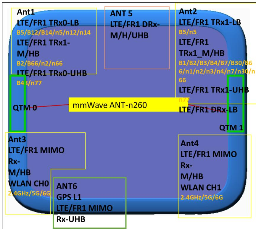
Figure 3 - 1: Netgear 5G MHS Travel Router (FCC ID: PY321100529) Antenna Block Diagram
