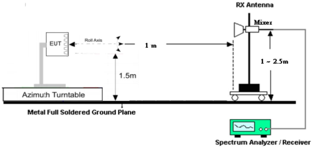
For radiated emissions above 140GHz up to 200GHz
