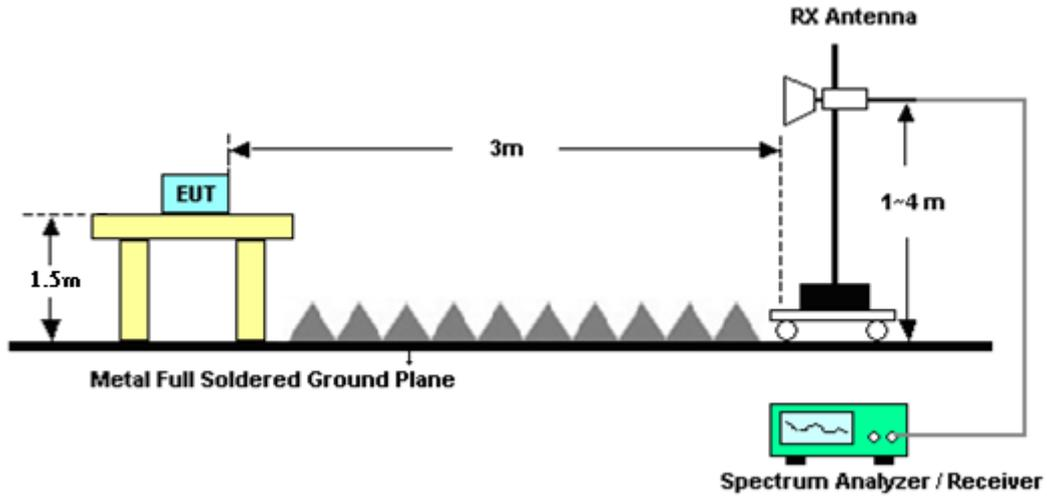
For radiated emissions above 18GHz up to 40GHz
