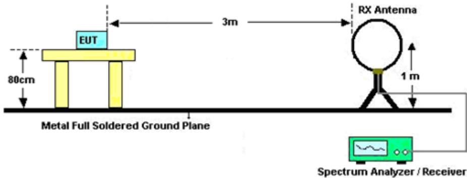
For radiated emissions from 30MHz to 1GHz
