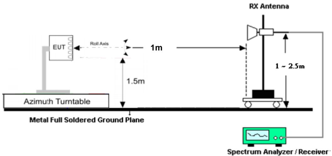
For radiated emissions above 40GHz up to 140GHz
