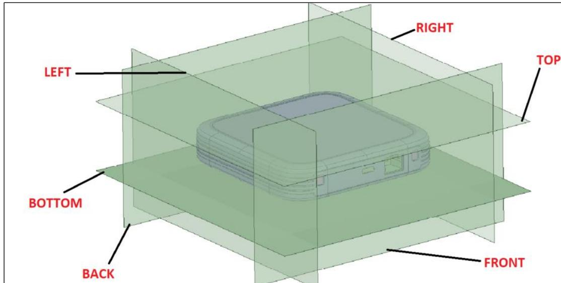
Figure 4 - 1 Device surface definition: Six surfaces of EUT
