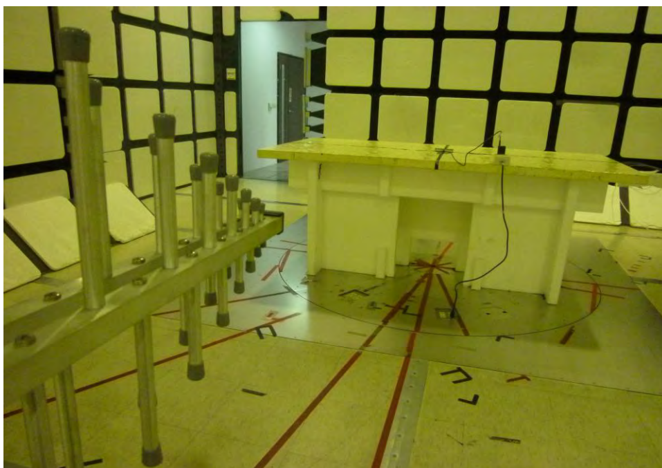
Below 1 GHz _ Rear View (AC Adapter : 2ACS005B)
