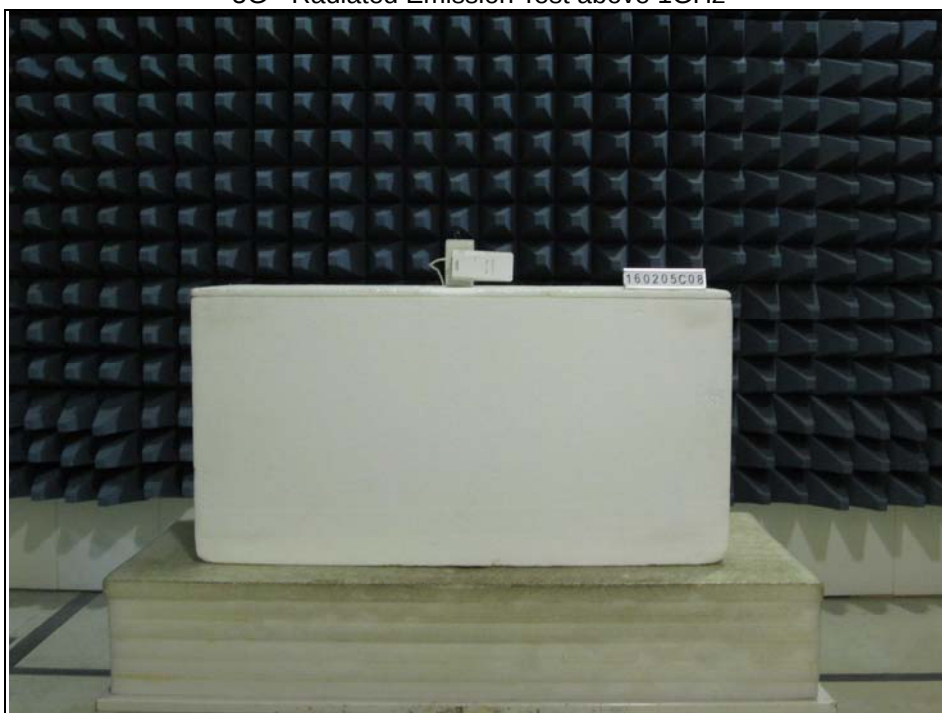
5G - Radiated Emission Test above 1GHz
