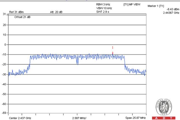
**4.6 Conducted Out of Band Emission Measurement**
