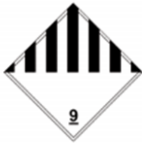
Figure143. Class 9 Hazard Symbol shipping label for batteries contained in the equipment.
