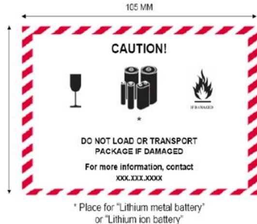
Figure 13: Shipping Labels for Smaller Packages for Batteries
