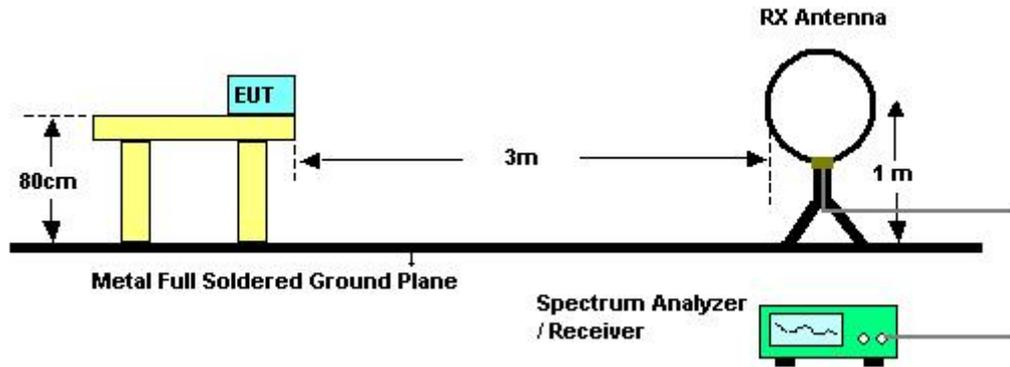
For Radiated Emissions: 30MHz~1GHz
