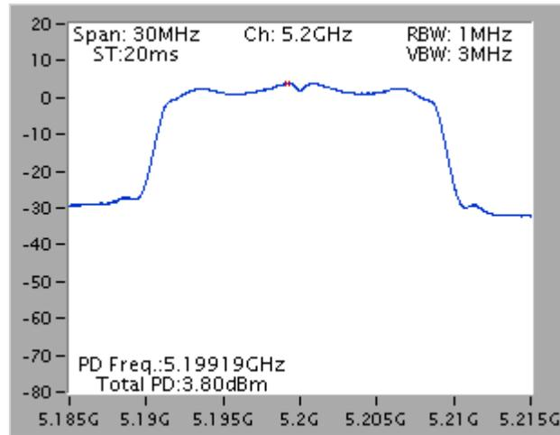
Power Density Plot on Configuration IEEE 802.11n MCS0 20MHz / Ant. 1 + Ant. 3 / 5230 MHz
