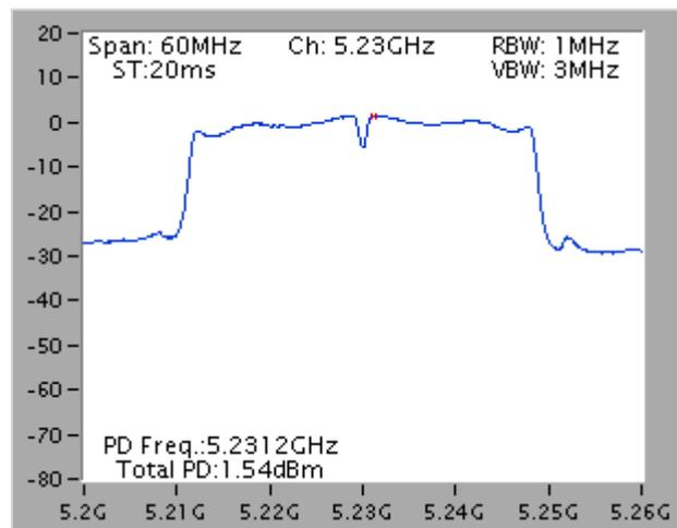
Power Density Plot on Configuration IEEE 802.11a / Ant. 1 + Ant. 3 / 5200 MHz
