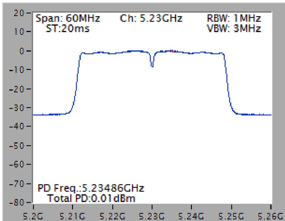
Power Density Plot on Configuration IEEE 802.11ac MCS0/Nss1 VHT 80MHz / Chain 1 + Chain 2 + Chain 3 / 5210 MHz
