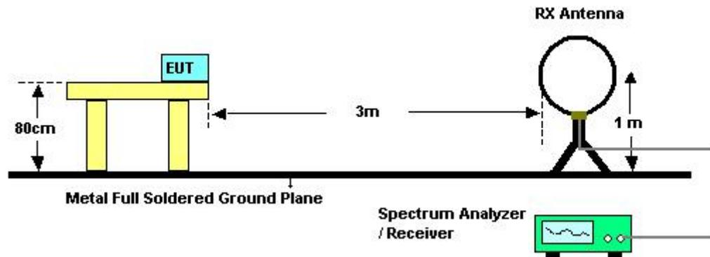
For Radiated Emissions: 30MHz~1GHz
