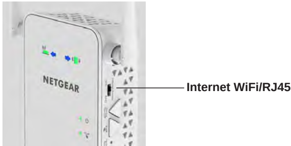
Figure 4. Internet connection switch
