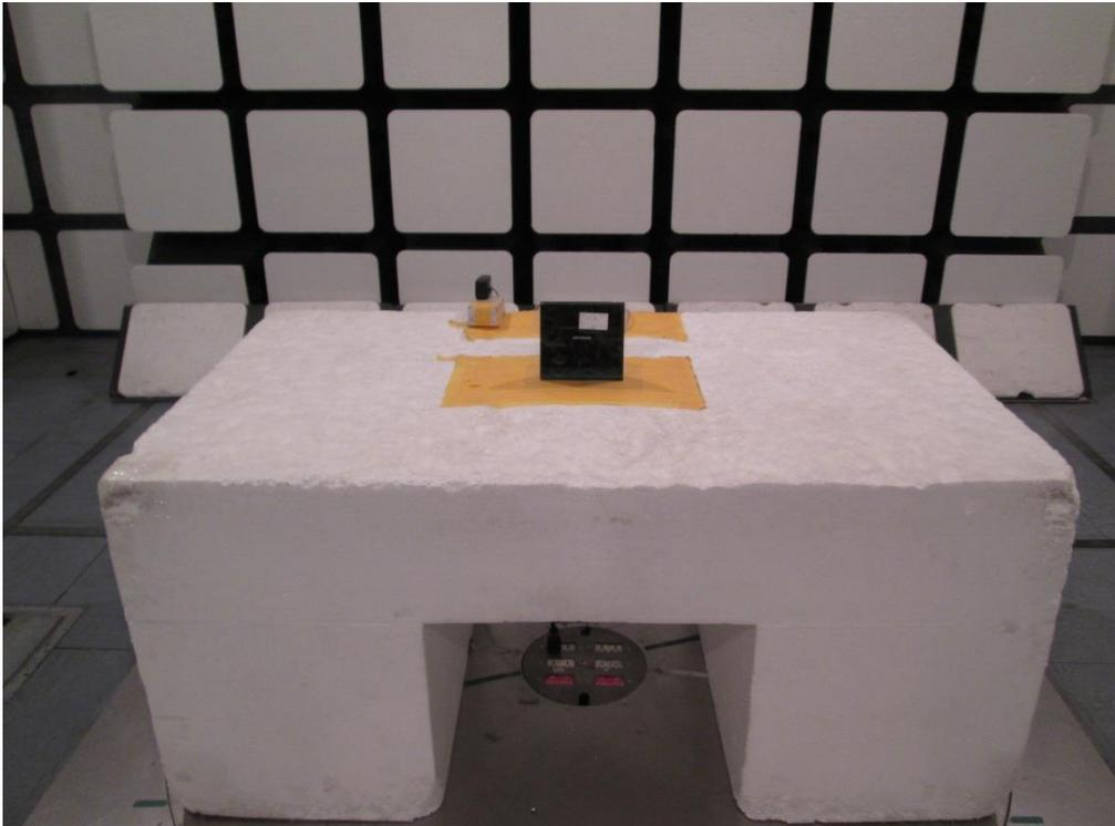
Radiated Above 1GHz Test
