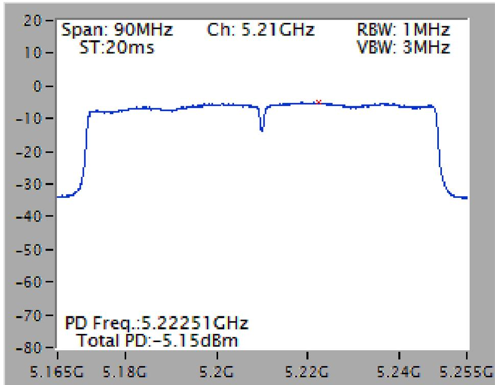
Power Density Plot on Configuration IEEE 802.11a / Chain 3 + Chain 4 / 5240 MHz
