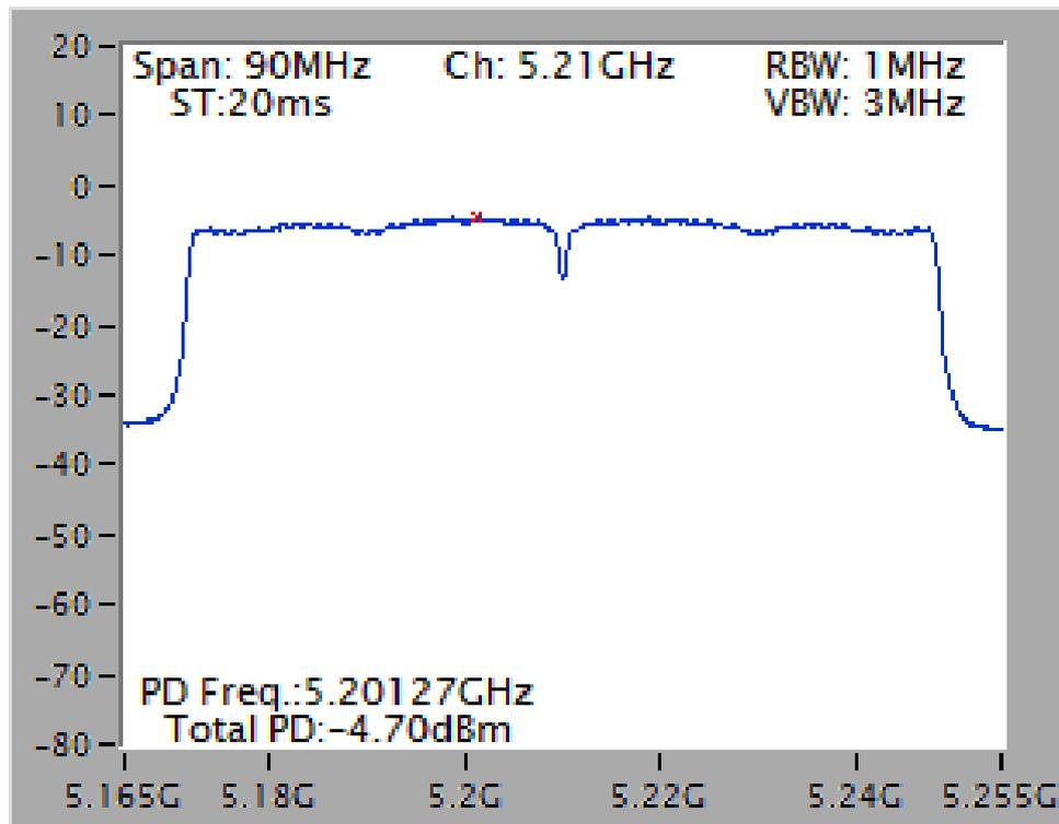
Power Density Plot on Configuration IEEE 802.11a / Ant 3 / 5240 MHz
