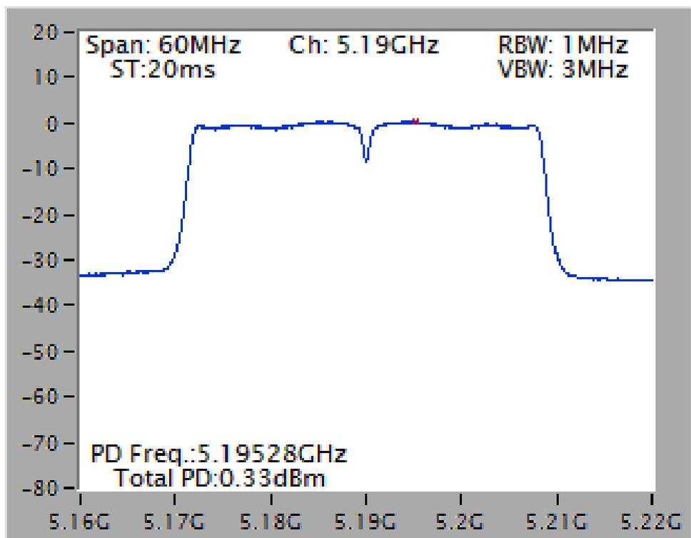
Power Density Plot on Configuration IEEE 802.11ac MCS0-Nss2 VHT 80 / Ant 3 + Ant 4 / 5210 MHz
