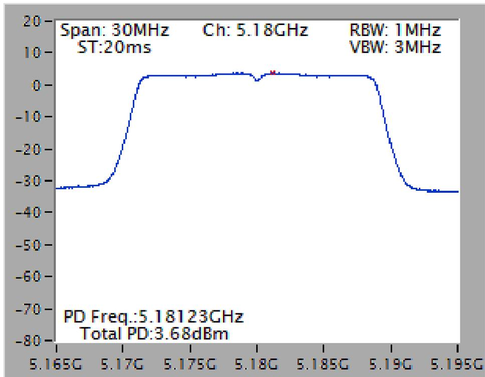
Power Density Plot on Configuration IEEE 802.11n MCS8 HT40 / Ant 3 + Ant 4 / 5190 MHz
