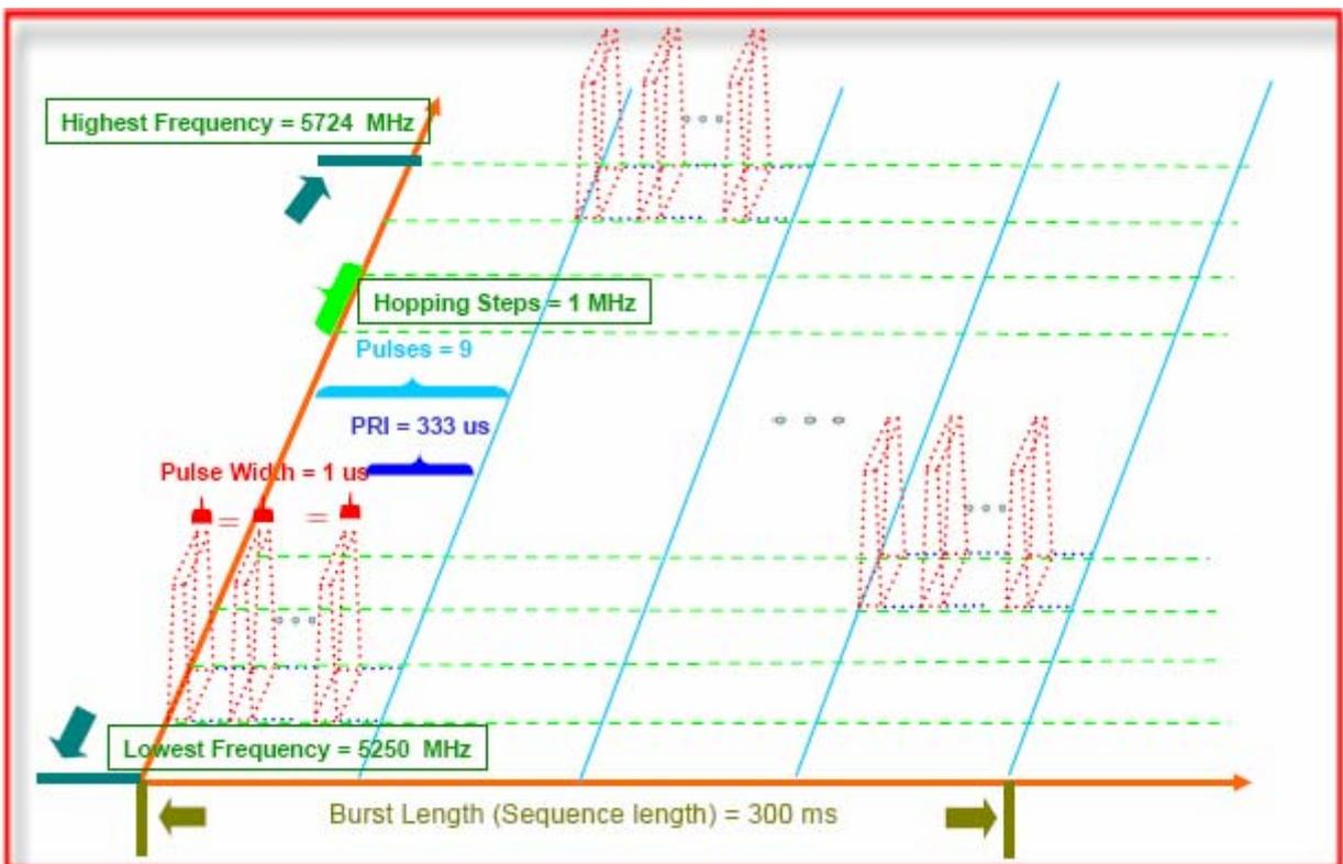
**Radar Types (6) System Diagram**
