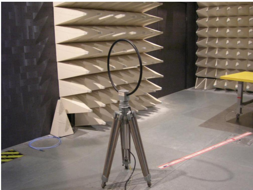
**For radiated emissions 30MHz~1GHz**
