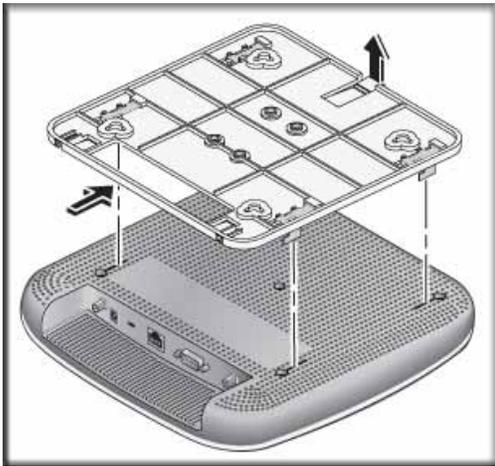
3. Attach the mounting plate to the wall.
