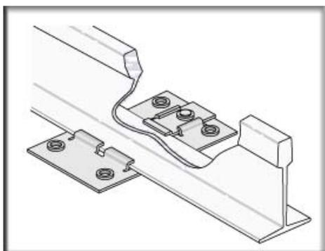
4. Attach the mounting plate to the clamp.
