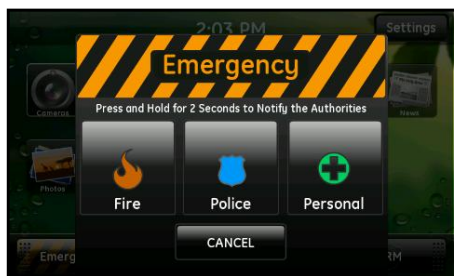
Figure 9. Fire, Police, and Personal emergency buttons
