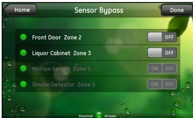
Figure 13. Choose sensors to temporarily bypass
