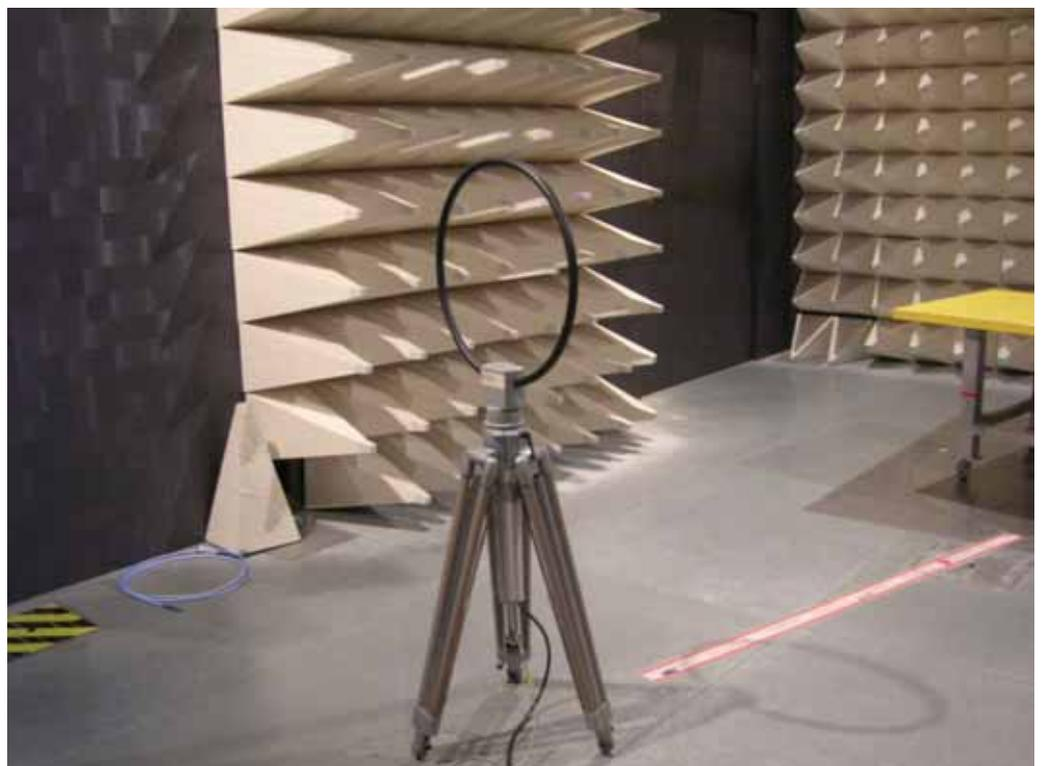
**For radiated emissions 30MHz~1GHz**
