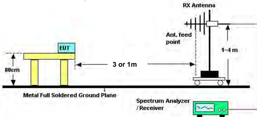
Above 10 GHz shall be extrapolated to the specified distance using an extrapolation factor of 20 dB/decade from 3m to 1m.
