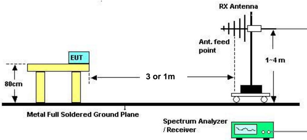
Above 10 GHz shall be extrapolated to the specified distance using an extrapolation factor of 20 dB/decade form 3m to 1m.
