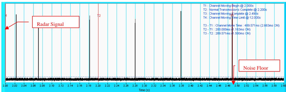
**NOTE:** An expanded plot for the device vacates the channel in the required 600ms
