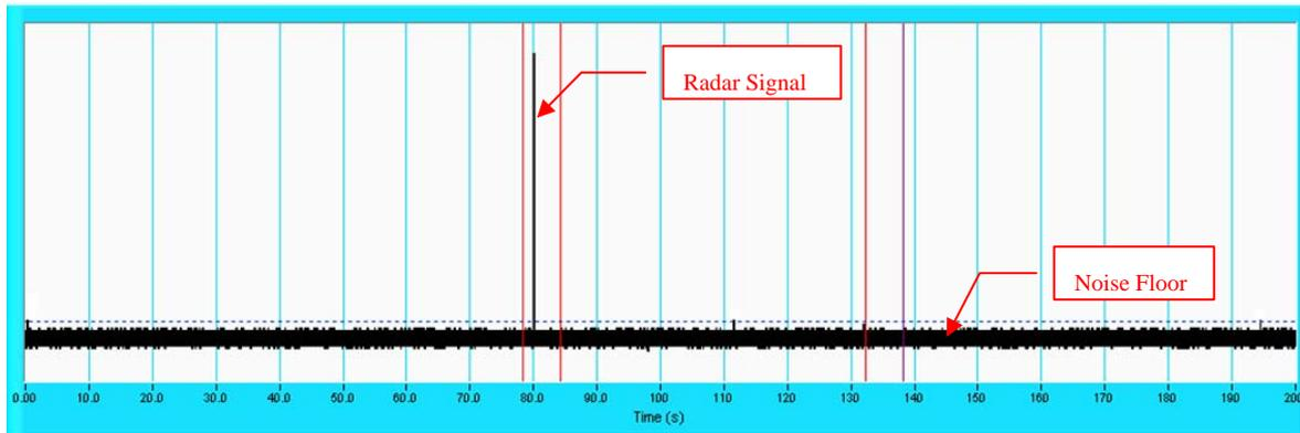
**NOTE:** T1 denotes the end of power up time period is 78 second. T2 denotes 84 second; the radar burst was commenced within a 6 second window starting from the end of power-up sequence. T4 denotes the 138 second.
