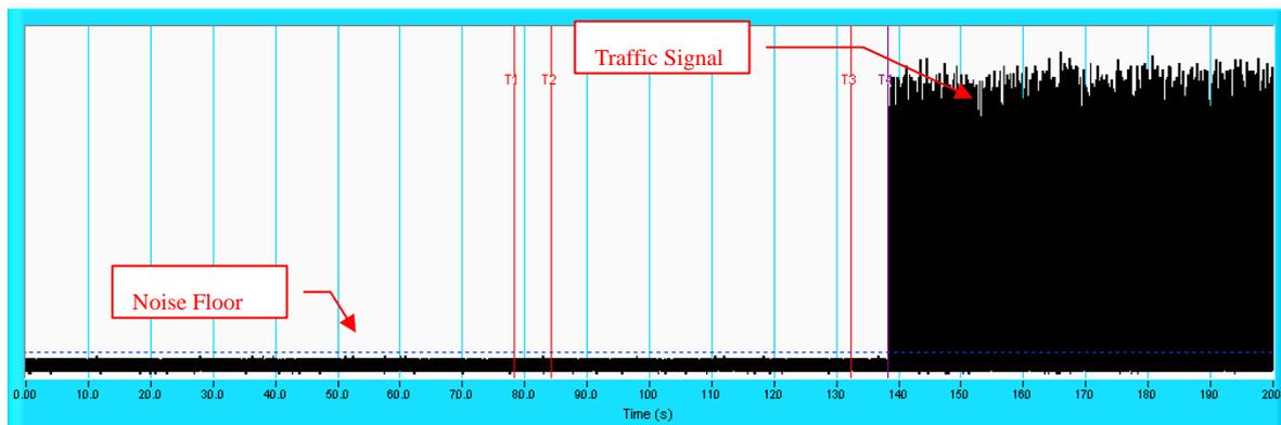
**NOTE:** T1 denotes the end of power-up time period is 78 second. T4 denotes the end of Channel Availability Check time is 138 second. Channel Availability Check time is equal to ( T4 – T1) 60 seconds.
