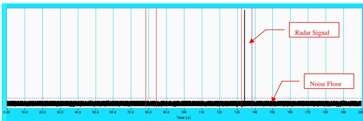
**NOTE:** T1 denotes the end of power up time period is 78 second. T3 denotes 132 second and radar burst was commenced within 54<sup>th</sup> second to 60<sup>th</sup> second window starting from the end of power-up sequence. T4 denotes the 138 second.
